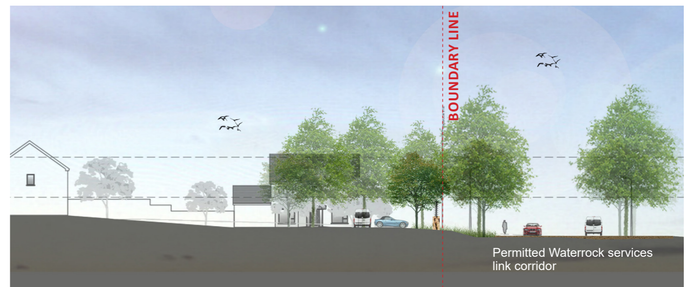
B - B' LOW NATURAL STONE WALL WITH A GALVANISED METAL RAILING, TOTAL HEIGHT C. 1.2M. GENTLY SLOPING TOPOGRAPHY WITH MOWN GRASS & WILDFLOWER MEADOW PLANTING.
