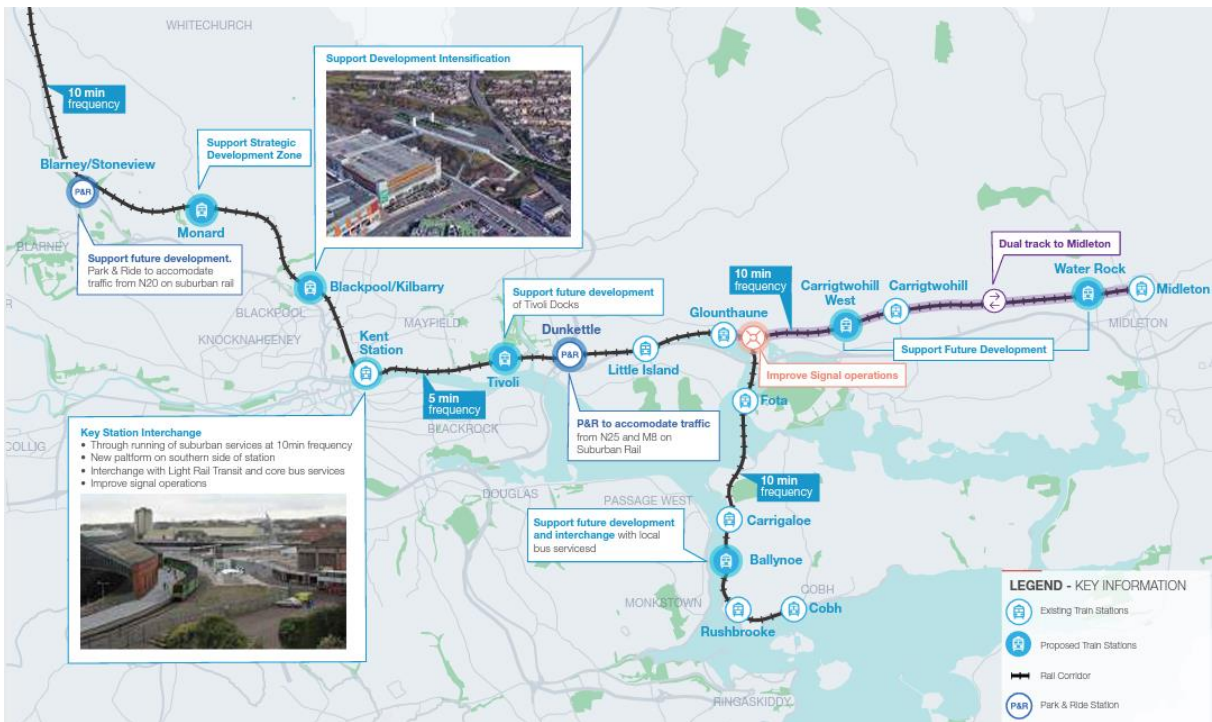
Figure 5.5: CMATS Proposed Suburban Rail Upgrades
