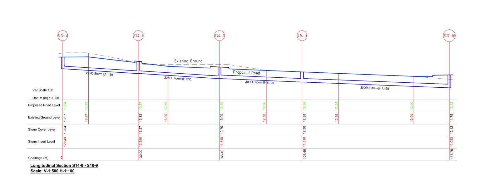
Proposed Road 225Ø Storm @ 1:30 Existing Ground 300Ø Storm @ 1:64 300Ø Storm @ 1:150 Ver Scale 100 \_\_\_\_ Datum (m) 10.000 Proposed Road Level Existing Ground Level Storm Cover Level Storm Invert Level Chainage (m)
